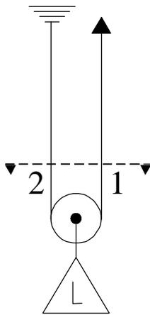
Cover the top half of the hauling system and count the number of lines attached to the load pulley. In this example (figure 4) the mechanical advantage is 2:1
