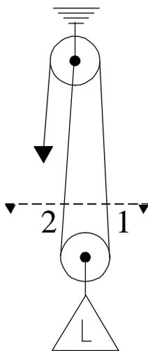
In this example (figure 5) the hauling line is not attached directly to the load. If you cover the top section of the hauling system you can see that only two lines are attached directly to the load pulley. The mechanical advantage of this system is still 2:1
